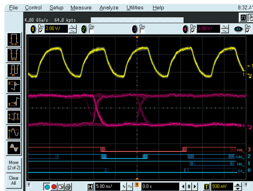
Figure 2. This six-channel measurement wouldn't be possible on a traditional DSO. A mixed-signal oscilloscope, however, enables the scope to trigger on a data “write” with RAS, CAS, WE, CS, and CLK using the 16 logic timing channels. The 4 scope channels are then freed up to evaluate signal integrity. The MSO used for this measurement is the 1 GHz Agilent 54832D.
